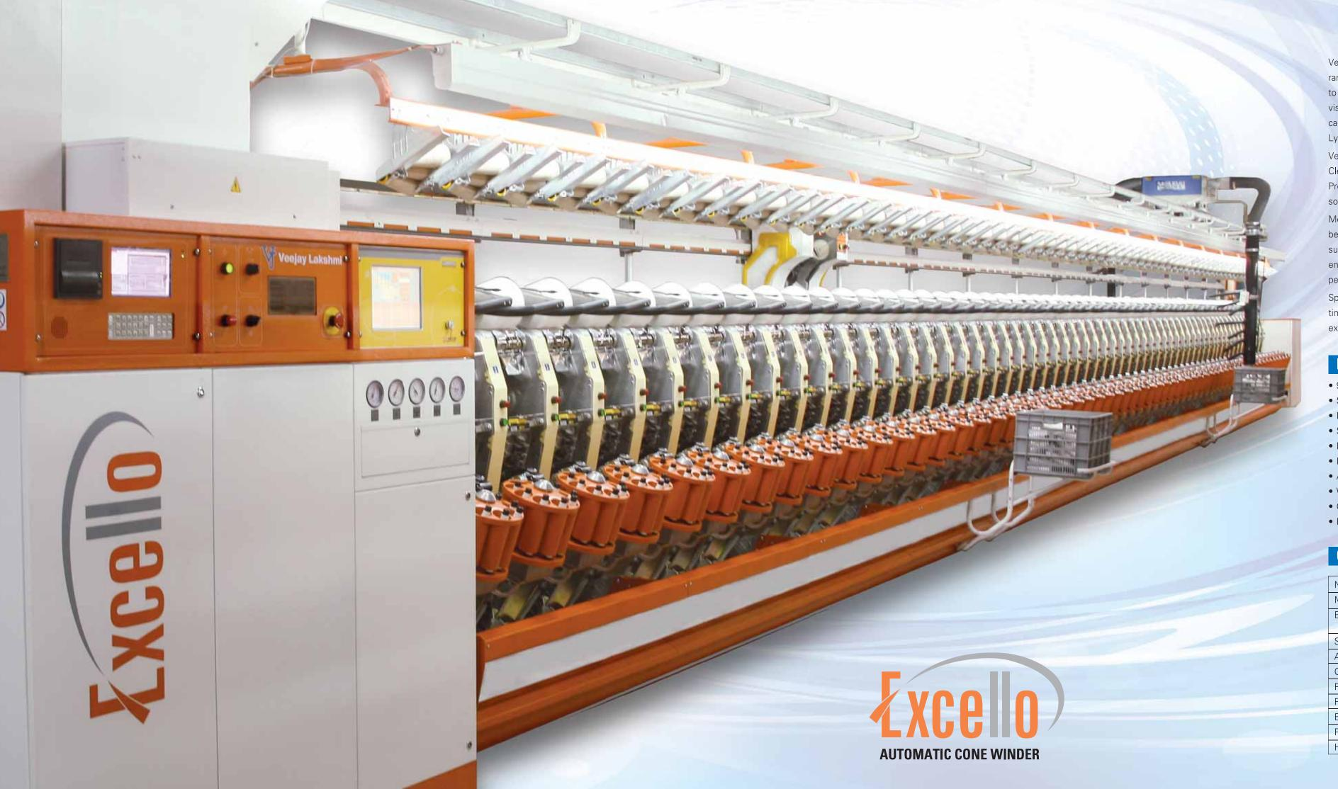
Veejay Excello Automatic Cone Winder is highly versatile in terms of count range and processing materials. It is suitable for winding yarns from Ne 4s to Ne 120s and can process most of the fibres namely cotton, polyester, viscose, acrylic, wool and their blends etc. In addition to the single yarns, it can also wind double yarns and other non conventional yarns like Slub yarn, Lycra core yarn etc., with exceptional package quality.
